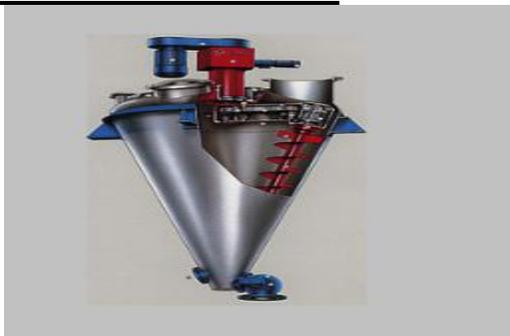
Cone screw mixer is widely used in chemical, food, cosmetic and pharmaceutical industries. The floor space required for this type of mixer is very less and they can be started on full load. The material of various densities, sizes and particle shapes are also mixed homogeneously without any degradation. The screw rotates about its own axis and revolves along the walls of the cone. Due to the conical shape the unloading of the material is helped by gravity and is complete without any hold-up.
