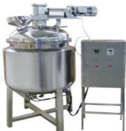
Reaction vessels are at the heart of a chemical plant. They are where the chemical changes and reactions take place. The capacity of reaction vessels can range from 50 liters to 250,000 liters and they are generally made from stainless steel, glass lined steel, glass or ceramics.
