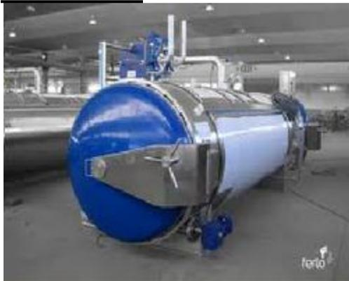
An autoclave is a device used to sterilize equipment and supplies by subjecting them to high pressure saturated steam at 121 °C for around 15–20 minutes depending on the size of the load and the contents.
