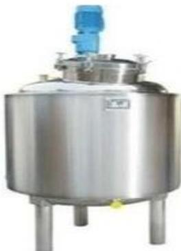
An agitator is a device or mechanism to put something into motion by shaking or stirring. There are three main types of agitation machines are as follow :
